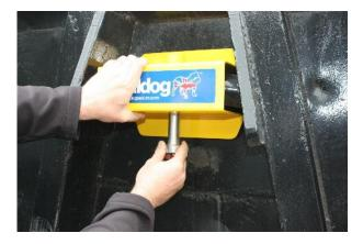
With the lock bolt in the unlocked position, insert it through the cover and lock it into the receiver by turning the key a quarter turn clockwise. Remove the key.
